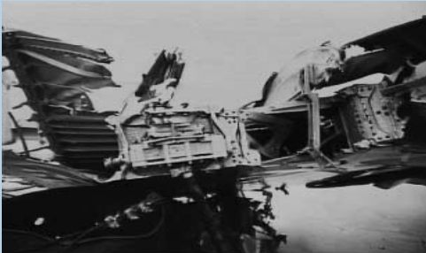
The jackscrew assembly of a MD-83 is recovered from the Pacific Ocean in 2000.
