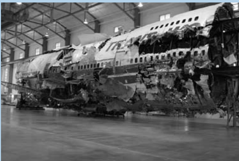
NTSB's goal to eliminate airliner fuel tank explosions is on the agency's Most Wanted List. Smoke rises from a fuel tank explosion in an aircraft parked at a gate in Bangkok, in 2001 (top photo). A tragic accident, attributed to an explosion of a fuel air mixture in center wing tank occurred on 1996 when a 747 crashed into the Atlantic Ocean, and claimed 230 lives. Reconstructing a portion of the downed plane aided NTSB investigators in finding the accident's probable cause. The reconstruction is housed at the NTSB Training Center and is used as a training tool for investigators.
