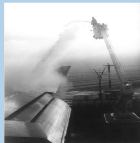
Deicing aircraft is a critical step in reducing the dangers of flying in icing conditions.
