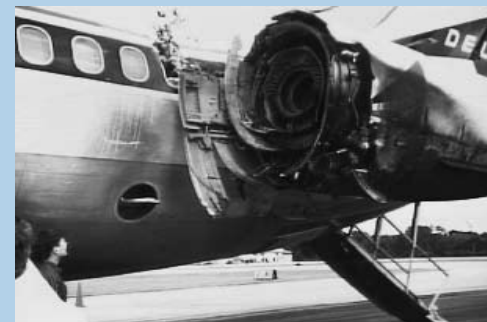
Debris from an engine that failed during takeoff punctured the cabin of a MD-88 in 1996, killing two passengers. Improvements in engine inspection and training resulted from the accident.
