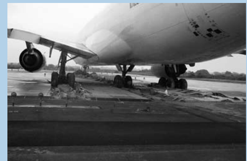
This cargo jet was stopped from running off the runway at New York’s LaGuardia airport in 2003. It was stopped by an “arrestor bed”—a cellular concrete structure at the end of the runway that slows the aircraft.
