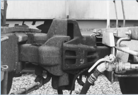
Tank car couplers were upgraded to prevent tank punctures. Couplers also help hold cars together during derailments.
