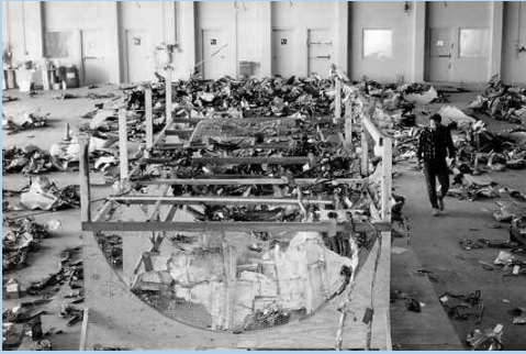
Reconstruction of the forward cargo hold of a DC-9 that crashed in 1996, killing all 110 on board, helped investigators determine the probable cause of the crash and make numerous recommendations that have been implemented to upgrade fire safety standards and hazardous materials rules and enforcement.
