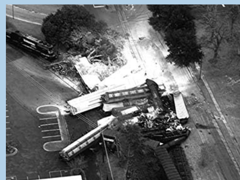
In 2005, the government reported that 90 percent of 203 railroad head-on, rear-end and side collisions were attributed to human factors causes. Implementing positive train control systems would have a major impact on reducing these types of accidents.
