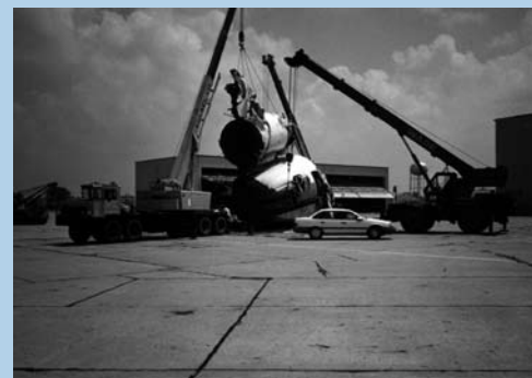
An uncontained failure in the engine on the tail of a DC-10 resulted in the loss of hydraulics and aircraft control.
