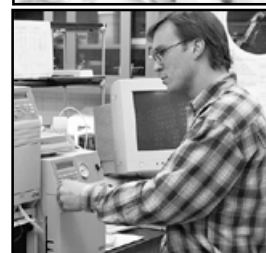
Scientist analyzing fatal aircraft accident specimen using high-performance liquid chromatograph.
