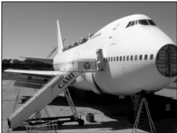
Evacuation Research Simulator. This retired Boeing 747 is now used for wide-body emergency evacuation studies.
