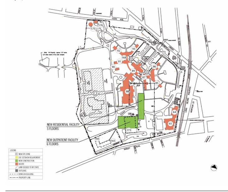
Figure 11: Proposed Site Plan – BPO 8: Construct New Outpatient/Clinic Building (Northwest Campus), Renovate Residential Building (Central Campus) by Linden Blvd.
