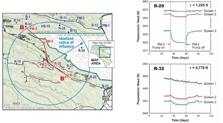
Pumping tests show the large radius of influence for municipal water supply wells, and large vertical anisotropy in the regional aquifer (kv << kh)</li>
