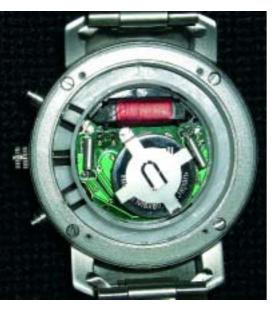
2. Rear view inside of a low-cost RCW, with two crystals and the antenna visible.
