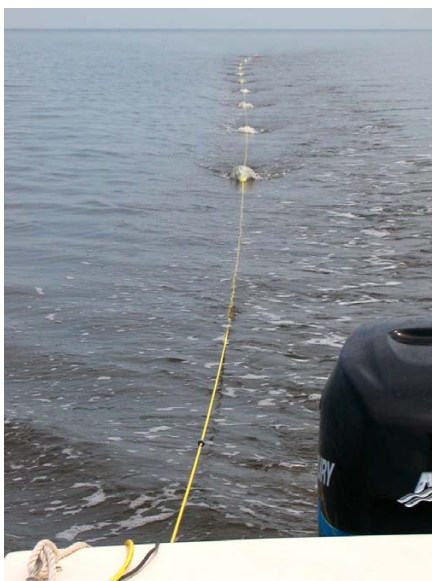
Electrical-resistivity streamer being towed behind the survey vessel.
