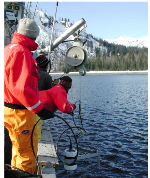
Guy Cochrane (left), Jodi Harney , and Jim de la Bruere (dark jacket) deploy a digital bed-sediment camera in Fingers Bay.
