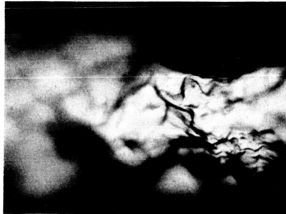
Figure II-10A, II-10B. Micro-Photograph of Tungsten Filament Eroded in a Glass Tube.
