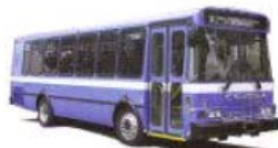
Standard Floor Transit Bus With a GVWR up to 35,000 lbs
