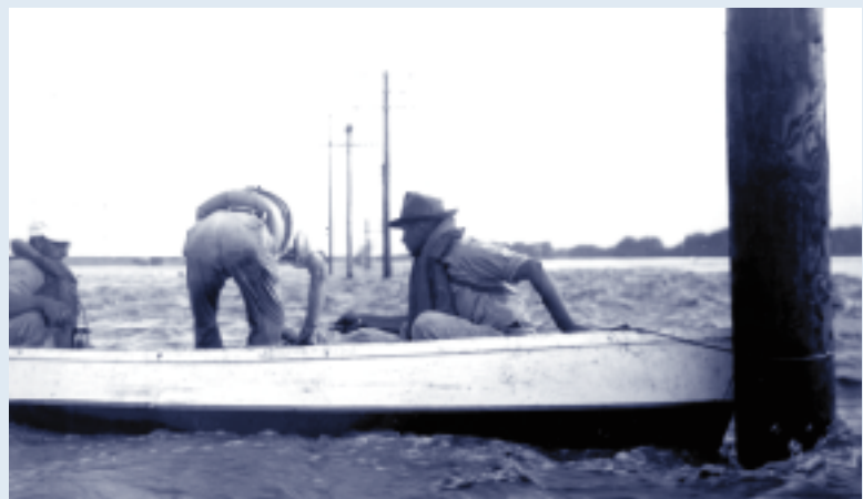
Figure 6. Overflow measurement by motorboat, Solomon River near Bennington, Kansas, July 14, 1951. It was necessary to secure the boat to the utility pole when the motor was turned off.
