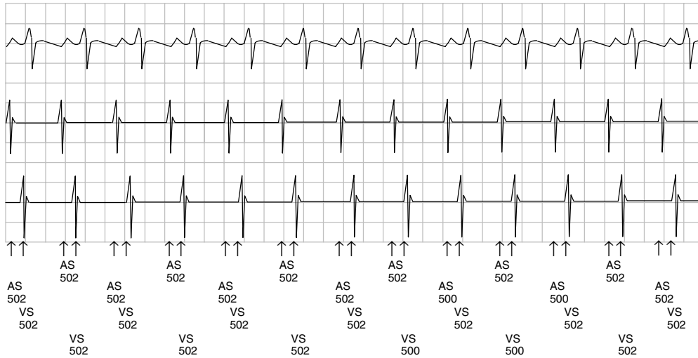
Figure 82. An example of annotated event markers and surface ECG as output on the programmer recorder. The numbers indicate the sensed heart rate (interval).
