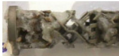
without micro mixer: fouling of the static mixer
