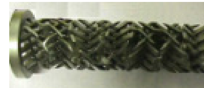
with micro mixer: no fouling
