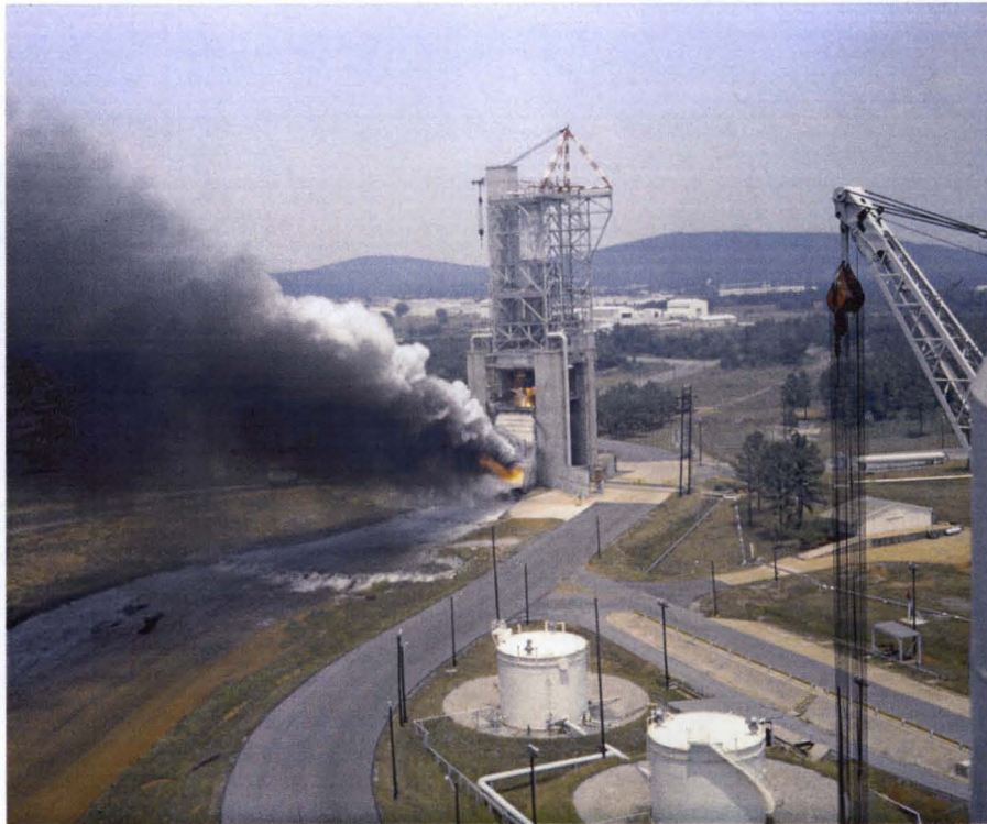
Fig. 3. Marshall's Static Test Stand accommodates large rocket engine testing, such as the Saturn V cluster of five F-1 engines.
