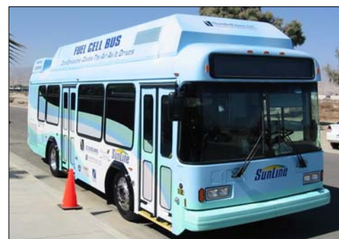
The prototype fuel cell hybrid bus from ISE Research uses a fuel cell by UTC.
