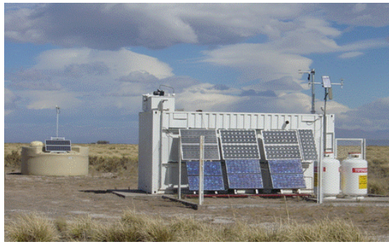
Figure 5. The central laser facility (CLF). The CLF is located near the center of the array, equidistant from three of the fluorescence detector enclosures. It can project a laser beam at angles from the horizon to the zenith at any azimuth for atmospheric monitoring and calibration checks. Light from the laser can be sent to the surface detector station in the background in order to make simulated hybrid events.
