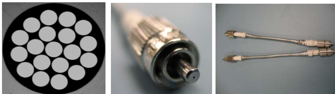
Figure 15: a) 200 X magnification of a 19 optical fiber array endface ferrule in an FC connector, b) Close up of FC ferrule and connector, c) 19 fiber custom array technology.
