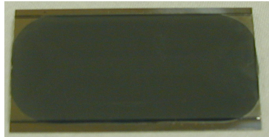
Epoxy test photo of glass readout board mockup glued onto blank Si (corners still need work)
