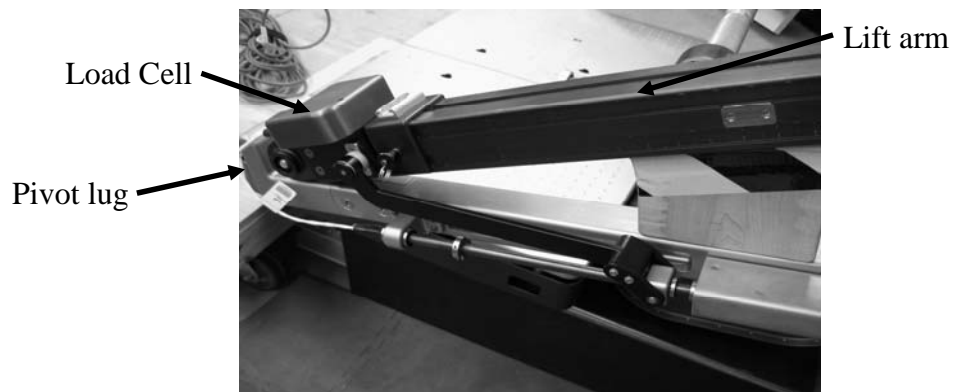
Figure 11. ARED lift arm shown with load cell and pivot lug.
