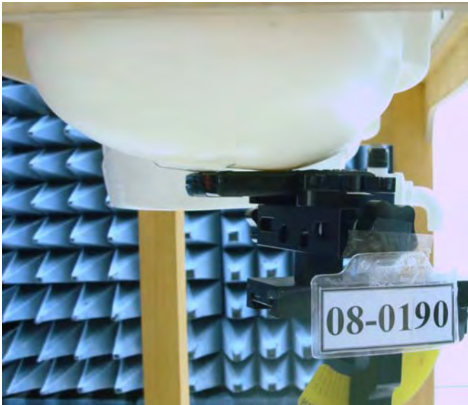
Figure 14. Right Head SAR Test Setup (Cheek)
