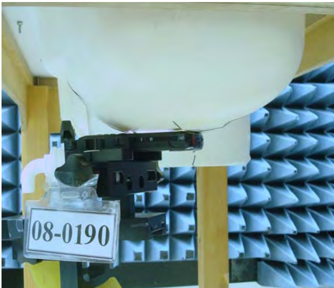
Figure 16. Left Head SAR Test Setup (Cheek)
