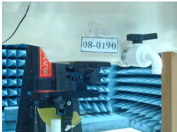
Figure 19. Body SAR Test Setup (Flat Section) _ 2 mm separation
