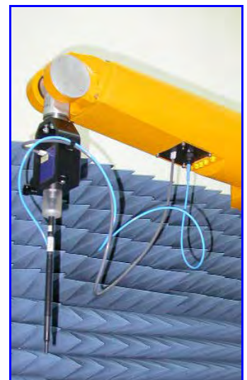
Figure 8. Probe setup on robot
