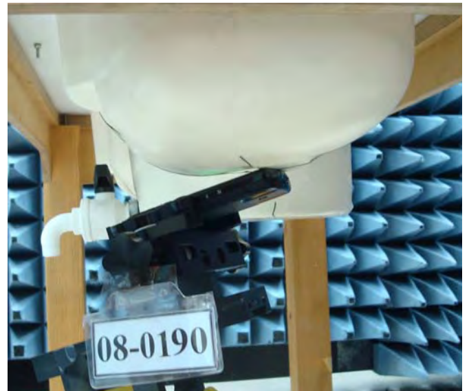
Figure 17. Left Head SAR Test Setup (Tilted)
