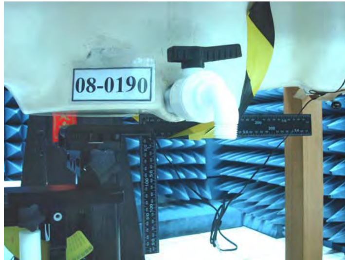
Figure 18. Body SAR Test Setup (Flat Section) _ 15 mm separation
