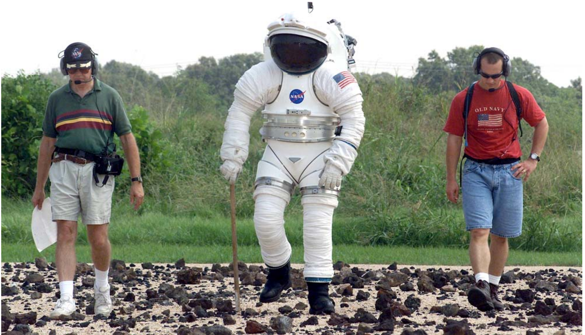
EC5 personnel conducting “dry run” suit mobility & communications testing at JSC prior to remote field activities
