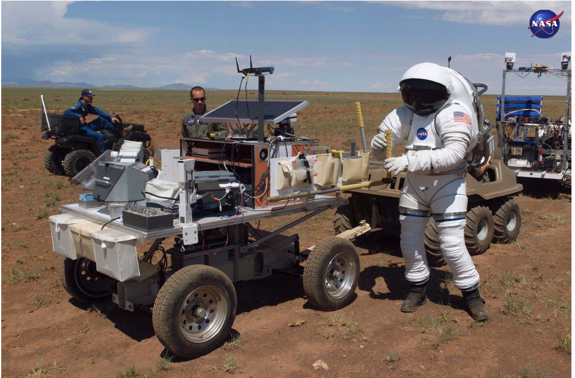
MK III suit subject conducting remote field site task activities with EC5 in-house developed Science Trailer (Mobile Geology Lab)
