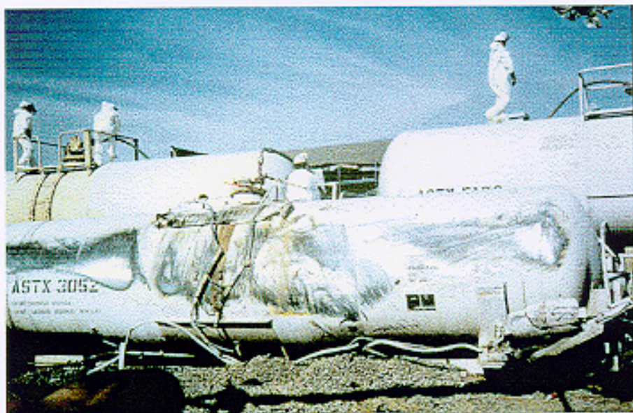
3-23D: These tank cars containing sulfuric acid derailed during the earthquake. Only one leaked.
