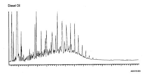
Figure 1. Chromatograms of Crude Oil and Diesel Oil, Showing Differences in the  $\rm C_{25}-C_{30}$  Range
