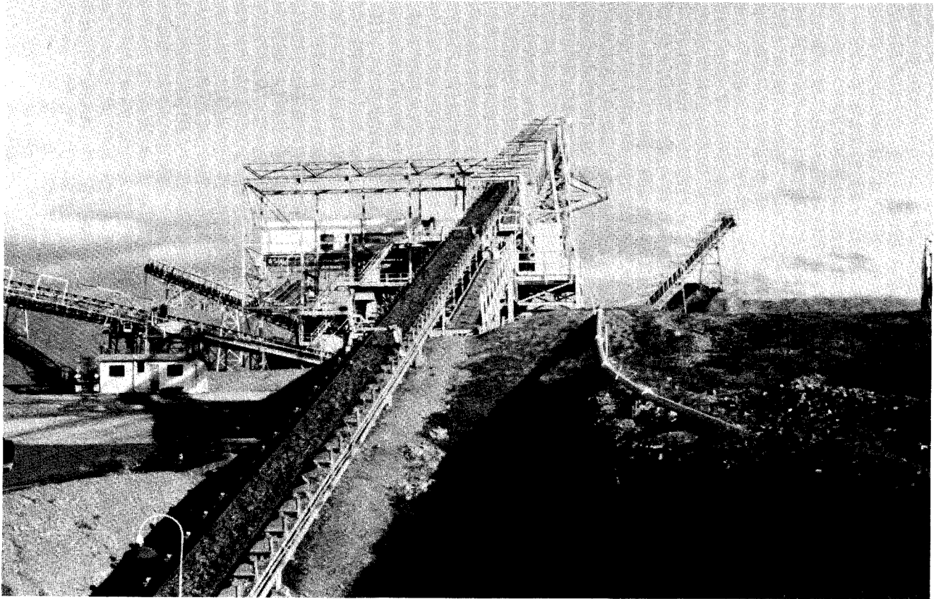
Figure 6. Example of aggregate-processing facility. Photo obtained with the cooperation of the National Sand and Gravel Association.
