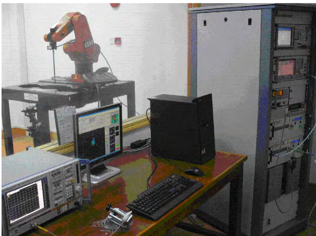
Figure B.1 COMOSAR Test Bench Test Layout
