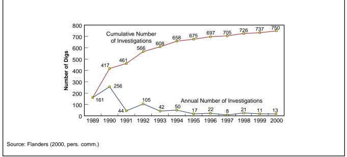
Figure 4.1-1. TAPS corrosion investigation projects for underground mainline pipe.
