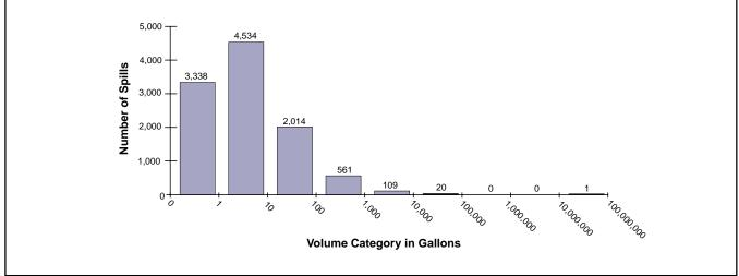
Figure 4.1-4. Number of spills by volume category (1977-1999). Total spills=10,577. Spills include ANS, TAPS, VMT, and marine transport.
