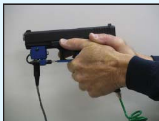
Dry fire with air-recoil system
