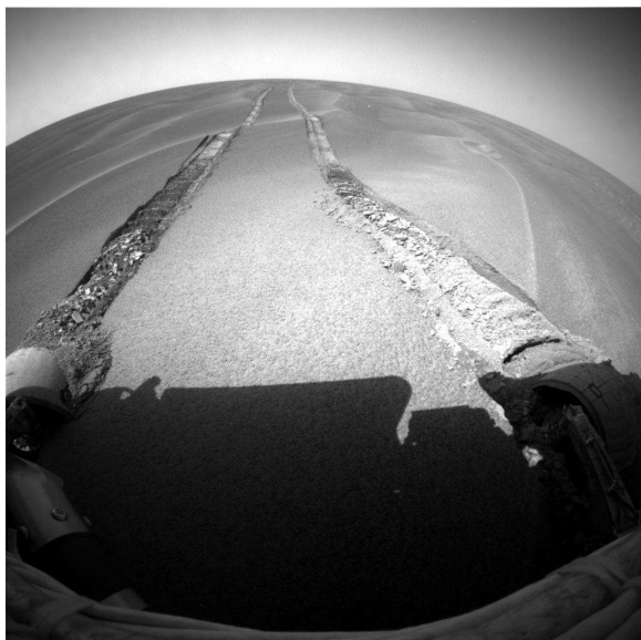
Figure 4. Front HAZCAM showing a non-geometric hazard encountered by Opportunity on Sol 446: 50 meters of commanded driving resulted in only 2 meters progress, which you can see in the tracks leading up to Purgatory Ripple, in which Opportunity was mired for over a month. Although this was a “blind” or Directed drive, Opportunity might have gotten stuck even if GESTALT had been turned on because there were no geometric hazards to avoid, just loose terrain. Fortunately, Visual Odometry has been used ever since as a Slip Check to ensure we never command more than 5 meters of driving without a guarantee of motion; this new safety check helped out on Sol 603, when Visodom measured 44% slip while climbing a similar dune, and stopped the drive before getting further bogged down. Opportunity was able to back out easily during its next drive.
