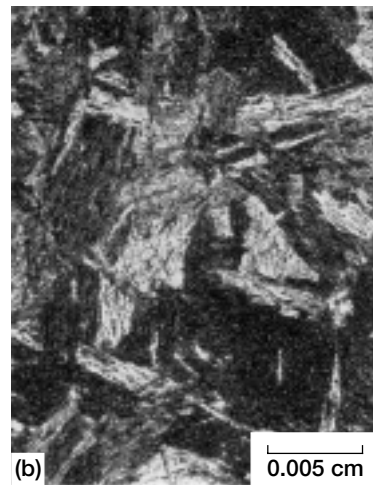
Figure 4.—Photomicrographs of case and core of AISI 9310 test gear. (a) Carburized and hardened case of the CEVM AISI 9310 gear showing high carbon fine grain martensitic structure. (b) Core structure of CEVM AISI 9310 gear showing low carbon refined austenitic grain size.
