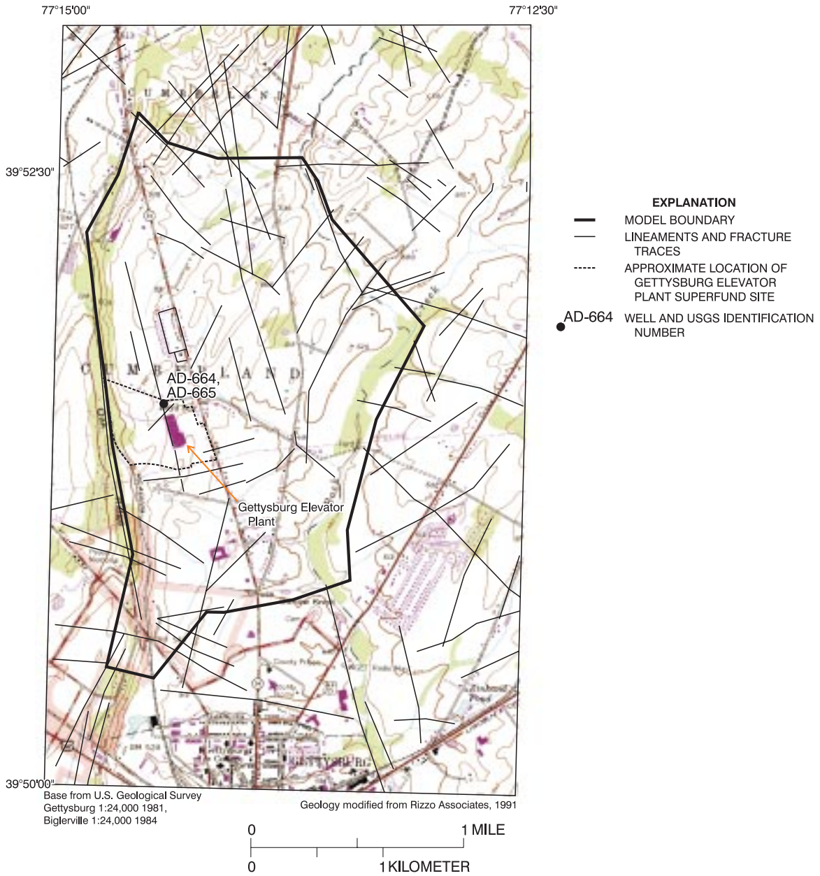
Figure 3. Location of fracture traces, lineaments, and selected wells in the vicinity of the Gettysburg Elevator Plant Superfund Site, Gettysburg, Pennsylvania (modified from Rizzo Associates, 1991).
