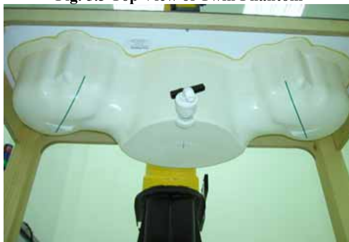
Fig. 5.4 Bottom View of Twin Phantom
