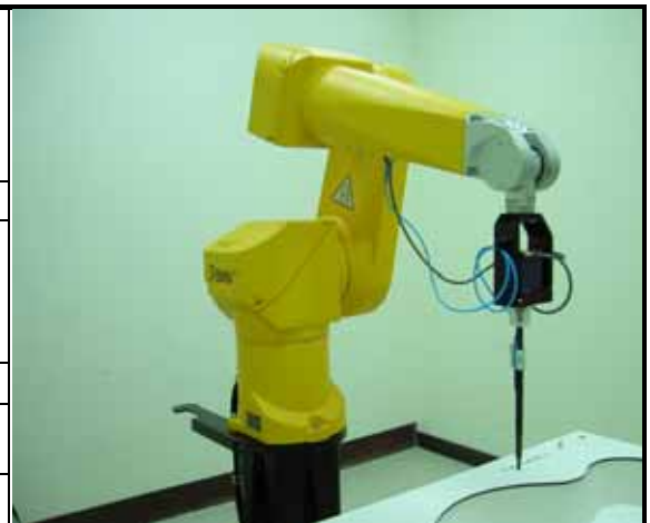
Fig. 5.2 Probe Setup on Robot
