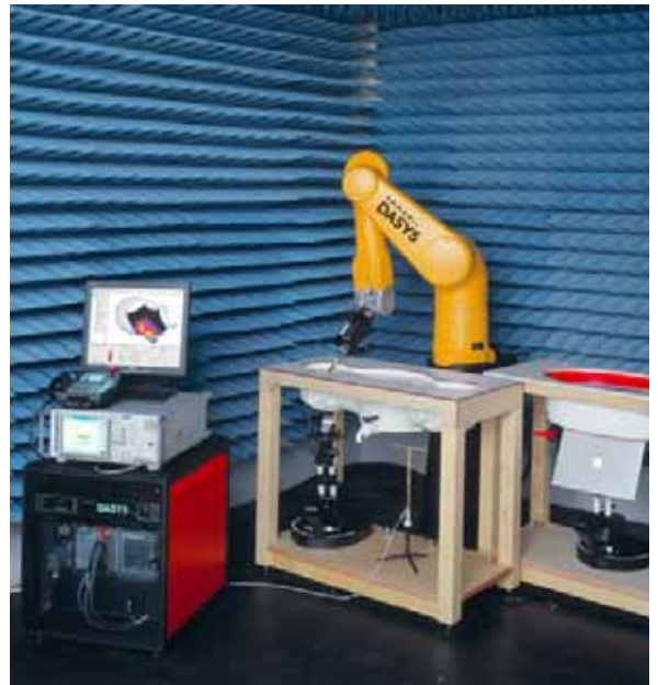
Fig. 5.2 Probe Setup on Robot
