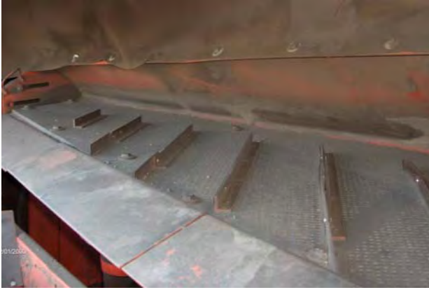
Left: Design of the FGX Air Table (table feeds right to left) Right: Separation of Product on FGX Table (right is clean coal, left is rock tailings)
