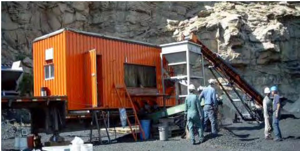
The FGX 5 tph Mobile Coal Deshaling Pilot Plant
