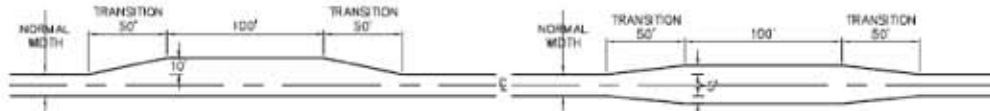
WIDEN SURFACE WIDTH AS SHOWN WHERE TURNOUTS ARE REQUIRED PLAN TURNOUT-WIDENING ON ONE SIDE (DETAIL)
