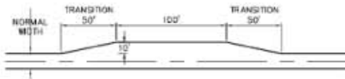
WIDEN SURFACE WIDTH AS SHOWN WHERE TURNOUTS ARE REQUIRED PLAN TURNOUT-WIDENING ON ONE SIDE (DETAIL)
