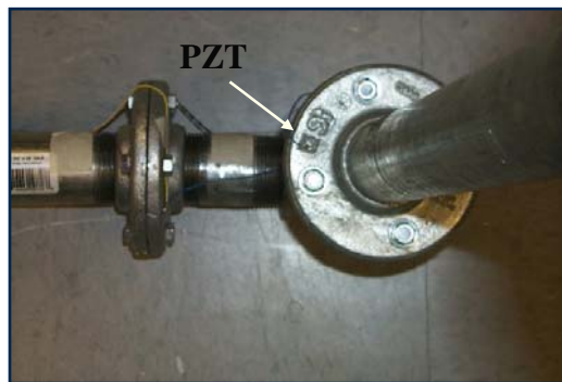
Figure 1: A piezoelectric patch attached to a bolted connection of a pipeline system
