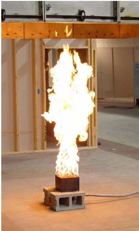
Figure 2. Natural gas calibration burner (HRR \approx 275 kW)
