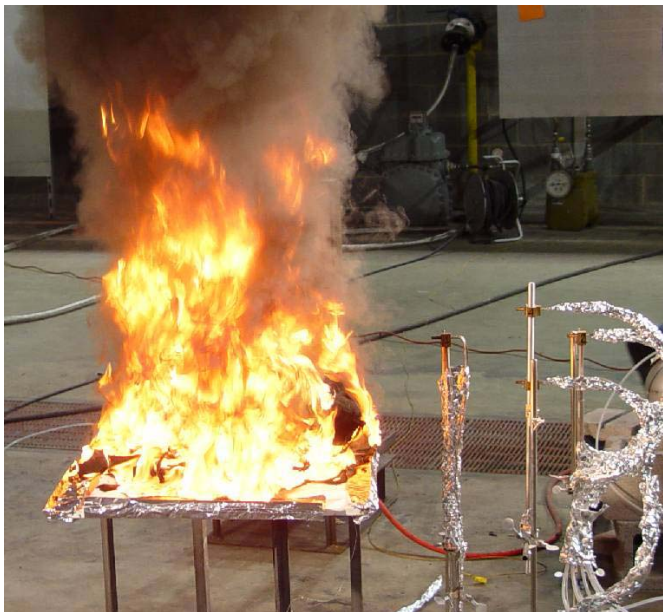
Figure 17. Image of monitor test #26, 3-HIPS-NFR, near peak heat release rate. Array of heat flux gauges is shown on right side of image.
