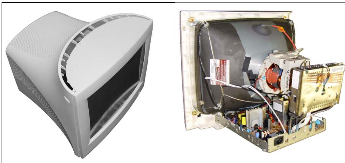
Figure 5. Photograph of 19” computer monitor test specimen. A 19” CRT is shown on the right side mounted to the front bezel.
