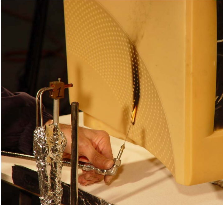
Figure 7. Needle flame ignition of 19" monitor specimen.
