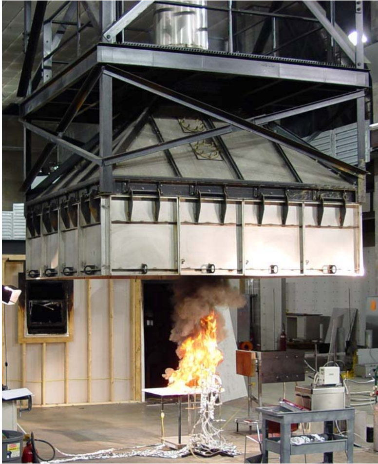
Figure 14. 3-HIPS-NFR monitor test #4, simulated internal components. HRR=155 kW, 7.5 min after ignition with needle flame.
