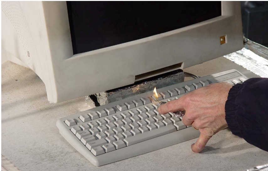
Figure 11. Keyboard ignition using 20 mm needle flame.
