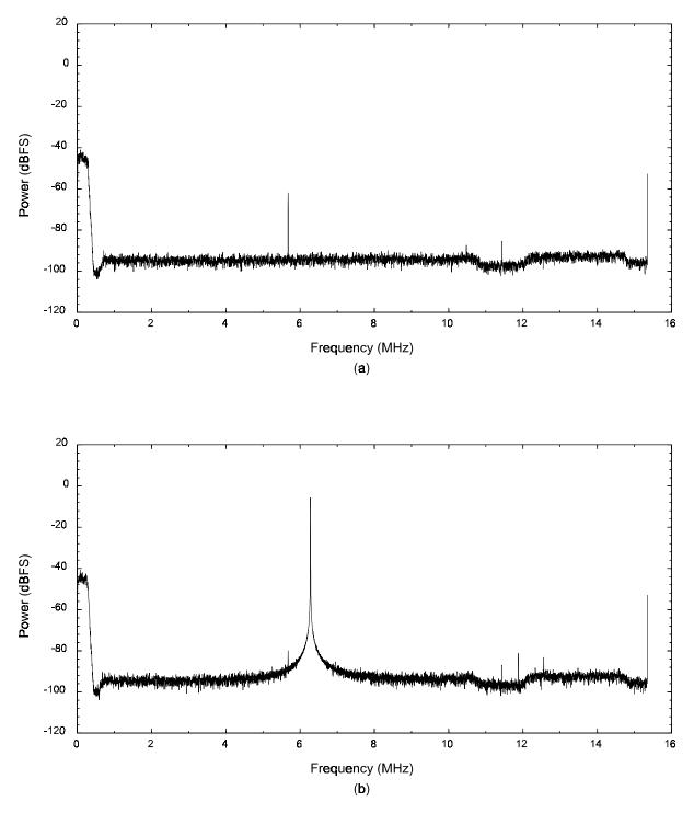
Figure 14. Averaged IF output power spectrum showing a low-level desired signal in the presence of (a) no interferer and (b) a high-level (-15 dBm) interferer.
