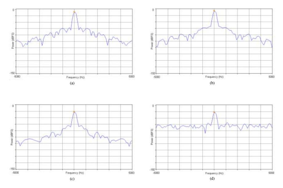
Figure 18. Output baseband spectrum with digital AGC enabled for 840-MHz RF input signal levels of (a) -15, (b) -40, (c) -60, and (d) -110 dBm.
