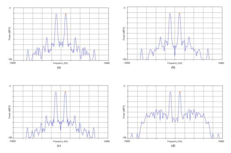
Figure 20. Demodulated output signal spectrum with digital AGC enabled for 840-MHz RF input signal levels of (a) -15, (b) -40, (c) -60, and (d) -110 dBm.
