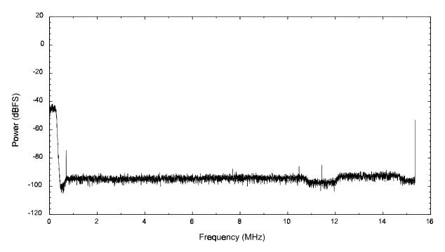
Figure 10. Averaged IF output power spectrum for an 835.02-MHz, -110 dBm RF input.
