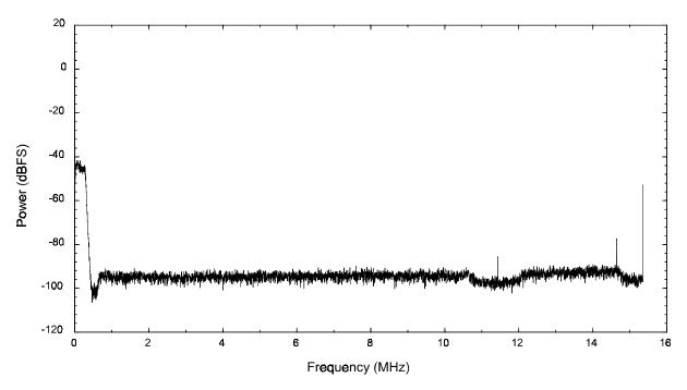
Figure 12. Averaged IF output power spectrum for the in-band aliasing test.
