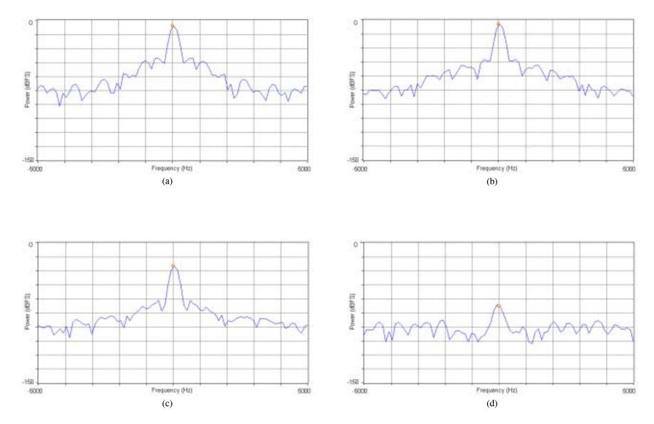
Figure 19. Output baseband spectrum with digital AGC disabled for 840-MHz RF input signal levels of (a) -15, (b) -40, (c) -60, and (d) -110 dBm.
