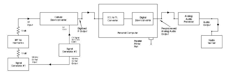
Figure 21. Test setup for the audio output channel desensitization test.
