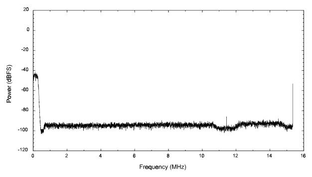
Figure 6. Self generated spurious response averaged power spectrum.
