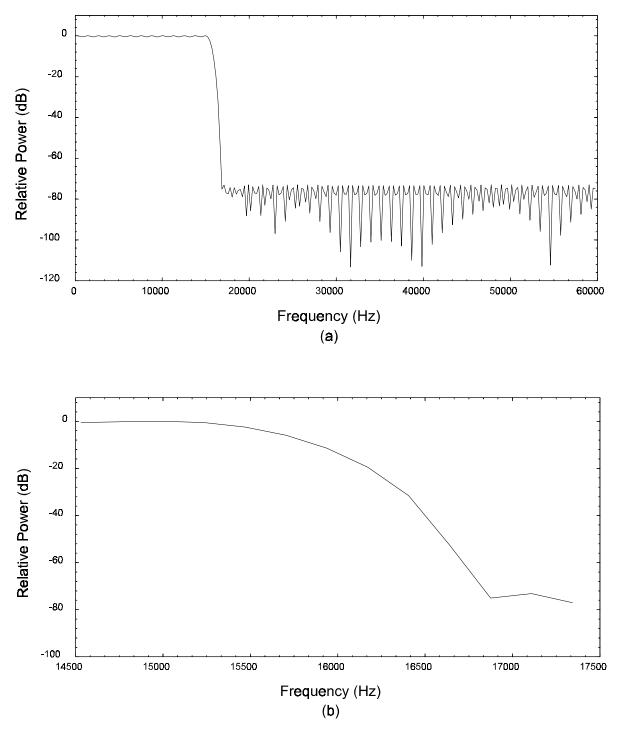
Figure 4. Magnitude response of the baseband FIR filter showing the (a) passband and stopband and (b) transition band.
