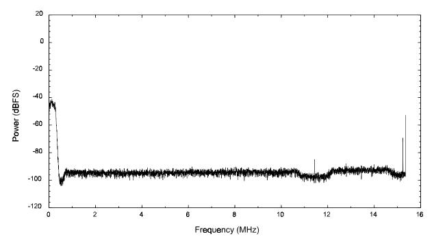
Figure 11. Averaged IF output power spectrum for the out-of-band aliasing test.
