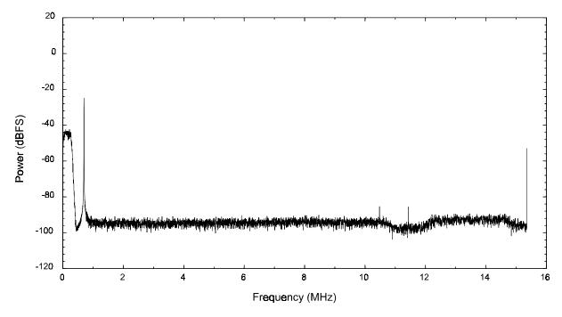
Figure 9. Averaged IF output power spectrum for an 835.02-MHz, -60 dBm RF input.
