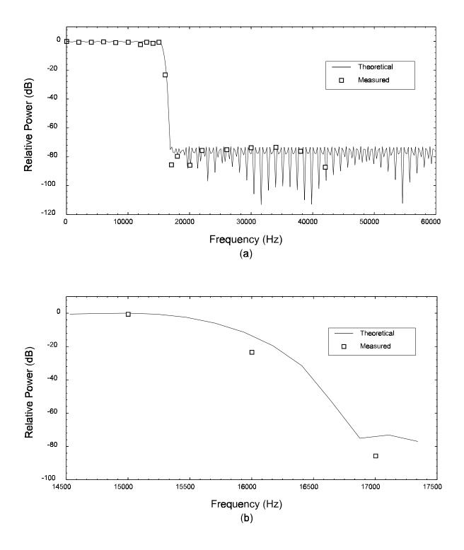
Figure 17. Measured and theoretical (a) passband and stopband and (b) transition band frequency response of the channel filter.
