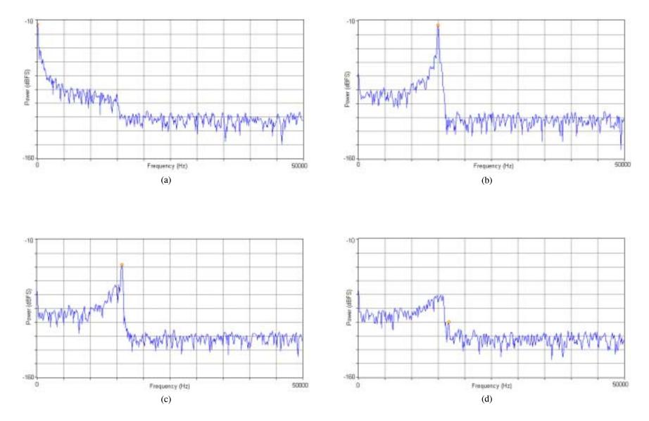
Figure 16. Example baseband output spectrum plots for determining the channel filter response at (a) 0 kHz, (b) 15 kHz, (c) 16 kHz, and (d) 17 kHz.
