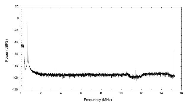
Figure 8. Averaged IF output power spectrum for an 835.02-MHz, -40 dBm RF input.
