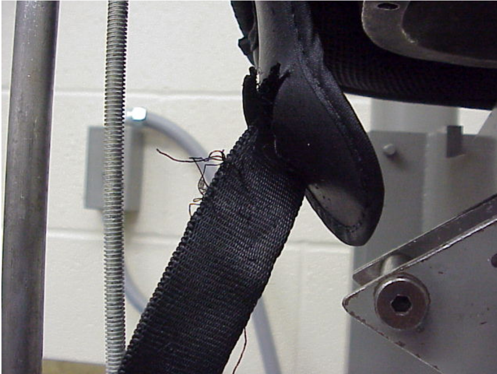
Helmet Photograph 11. Retention Water Immersed Vance Leather, 200, M
