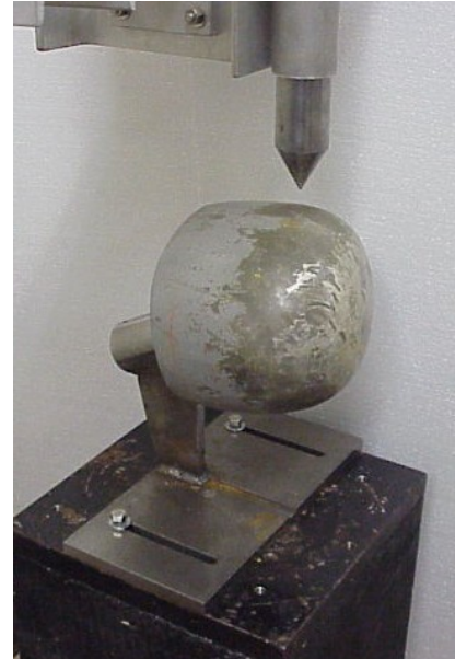
SwRI Helmet Test Equipment Photo 5. Penetration Resistance Tester Configured for Side, Front, and Rear Locations
