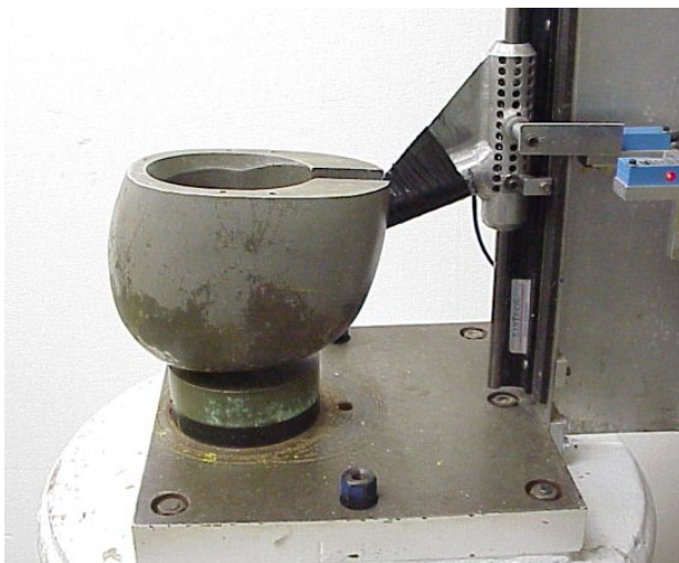
SwRI Helmet Test Equipment Photo 2. Flat Anvil Impact Configuration
