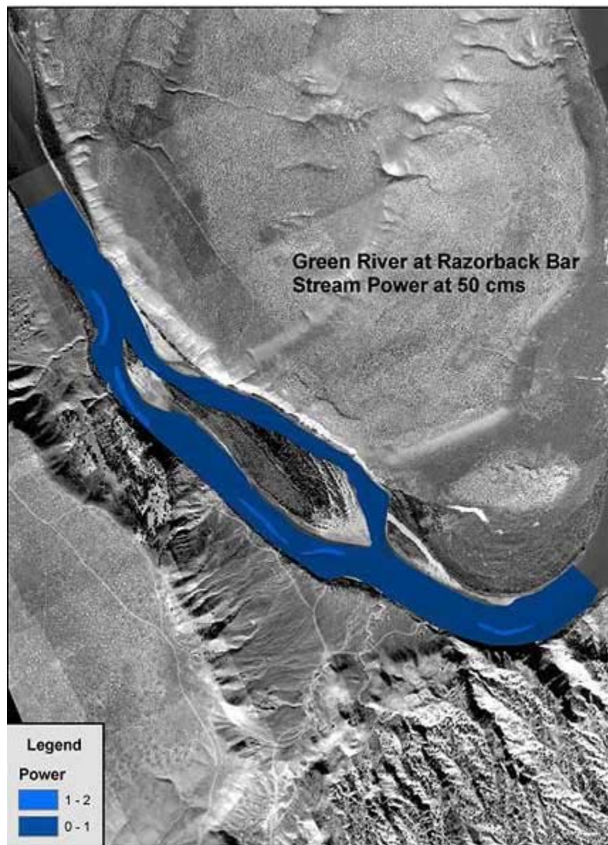
Figure C1. Stream power distribution in the Green River at 50 \text{ m}^3/\text{s} .
