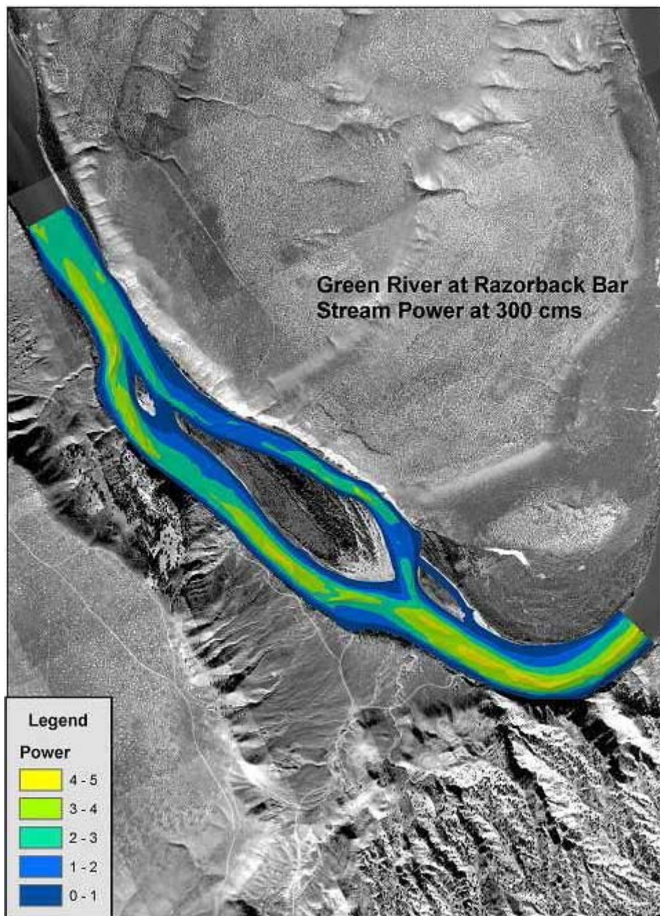
Figure C6. Stream power distribution in the Green River at 300 m 3 /s.
