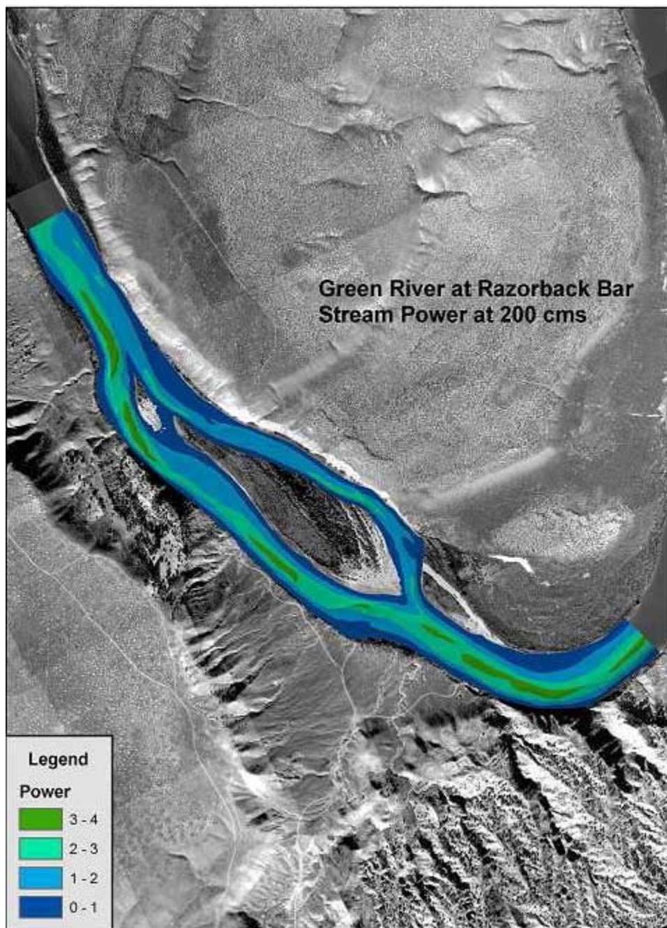
Figure C4. Stream power distribution in the Green River at 200 m 3 /s.
