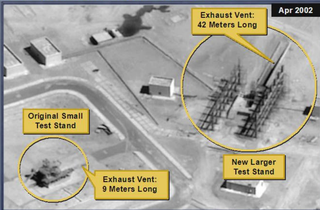
Test stand comparison Al-Rafa's Liquid Engine test facility. ( large image )
