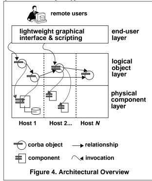
This architecture can be described in terms of how it supports integration—the core design activity in componentbased systems (architectural mismatch is the inhibitor of integration). One useful way to think of integration is as a *relationship* between two integrated entities, where the relationship has four *aspects*: control, data, process and presentation [9][10]:
