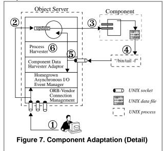
The core of the solution makes use of UNIX asynchronous I/O and sockets. The idea is to have the main event loop in the object server "listen" (via the *select()* system call) for activity on any number of socket connections, and when activity is detected on a socket invoke a callback procedure that is appropriate to the kind of activity detected (e.g., data avail-
