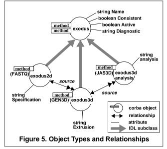
major object types and their relationships to each other and to the SEACAS components. For example, *exodus2d* (a twodimensional mesh) inherits (and defines its own) operations and attributes from the *exodus* abstract superclass; *exodus2d* functionality is implemented by *FASTQ*; and, it participates in a 1:many relationship with *exodus3d* objects to indicate that a single two-dimensional mesh can be extruded into several three-dimensional meshes.
