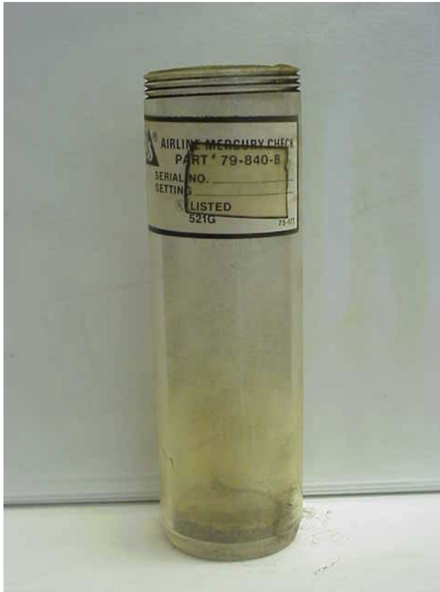
Device attaches to a plant air-line – partially filled with liquid mercury
