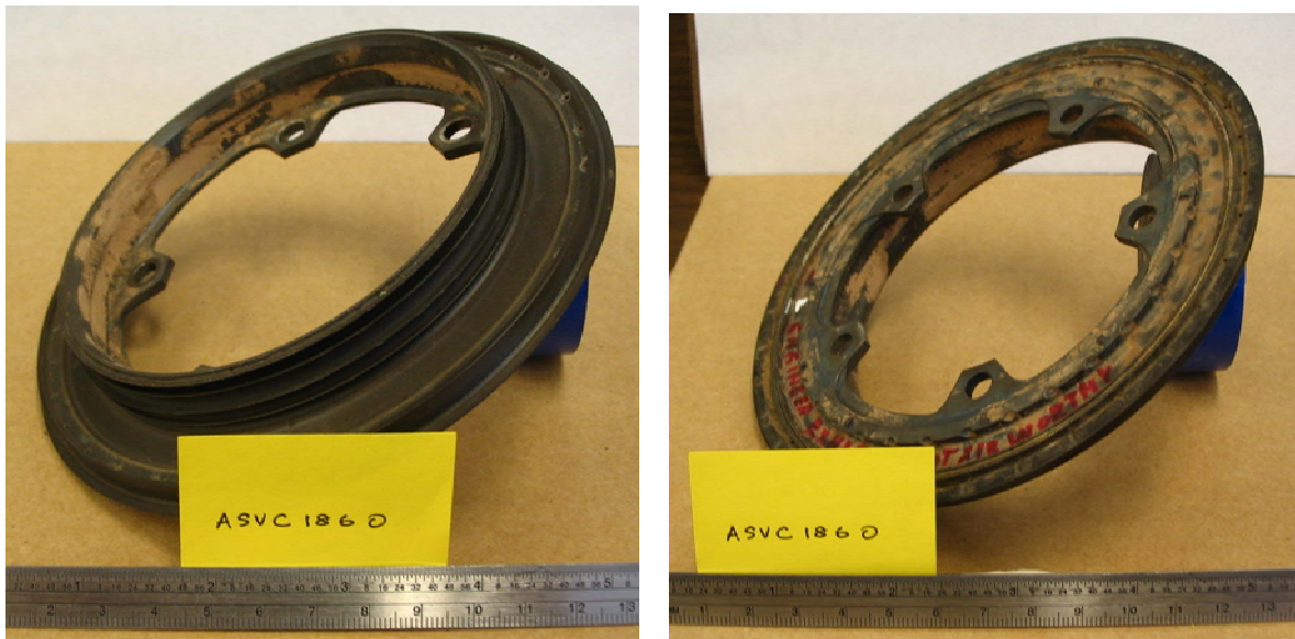
Figure 7.—Forward cooling plate with impacted sand.
