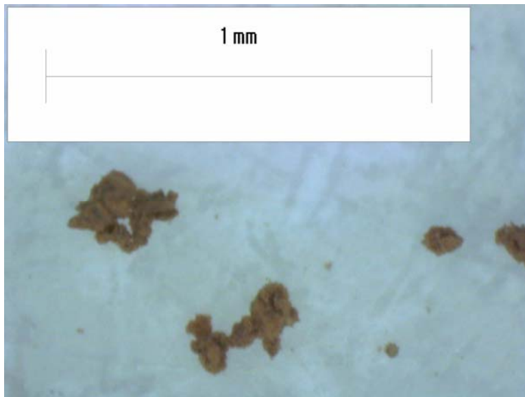
Figure 11.—Close-up micrograph sand particles from cooling plate, figure 7.
