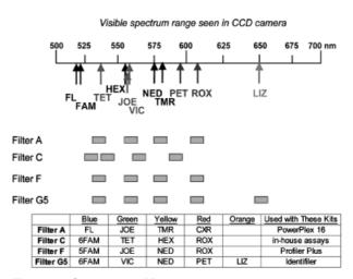
Figure 7. Schematic of fluorescent dye emission maxima and virtual filters used in ABI 310 with various STR kits.
