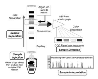
**Figure 2.** Schematic illustration of the separation and detection of STR alleles with an ABI Prism 310 Genetic Analyzer.
