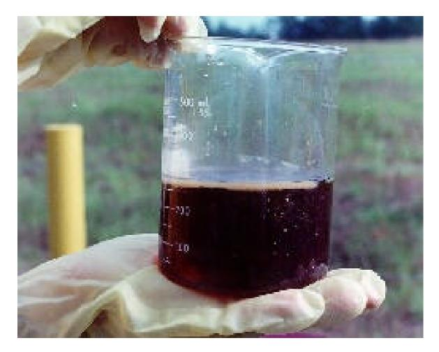
(Note: This is a worst-case example of extraction of free product from an aquifer well indicating mobile DNAPL from a vadose zone source. This sample consists of tetrachloroethylene, polychlorinated biphenol, and trichloroethylene in order of mass composition).
