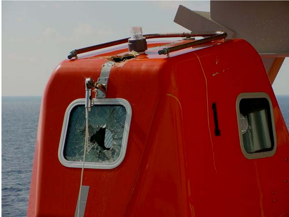
Figure 30 – Damage to Lifeboats at Typhoon
