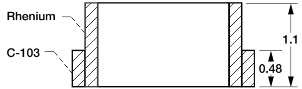
Figure 4.—Tubular coupon configuration. Dimensions in centimeters.
