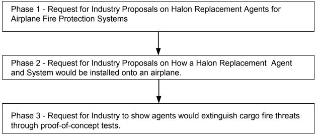
Figure 2. Phase Request for Cargo Fire Suppression Information.
