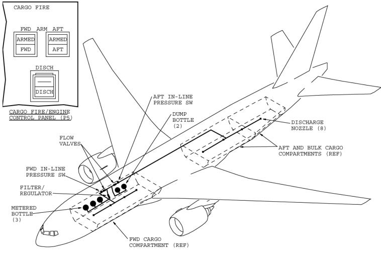
Figure 1. Typical Airplane Cargo Fire Suppression System Schematic.
