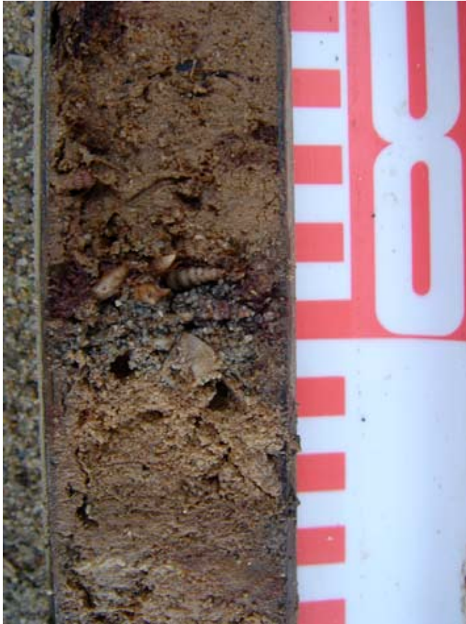
Figure 19. Core of sediments beneath wetlands at Bajura, Puerto Rico (Fig. 3, site 7) showing event deposit of sand and shells encased in laminated mud. Scale is in cm.
