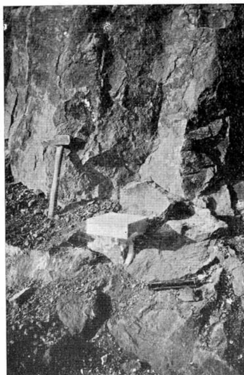
Figure 14. Method of orienting and collecting rock samples using a “plaster of Paris cap” (“chapeau de plâtre”) pioneered by E. Thellier [from Thellier , 1938, Figures 44 and 45].
