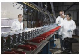
Level 2 manager Howard Budd observes as technician Dan Ruggiero, and technical associate Heng Bao Zeng, inject epoxy at the gluing station into optical connectors holding optical cables that will become part of the MINERvA detector.
