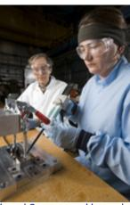
Level 2 manager Howard Budd watches as technical associate Janina Gielata puts epoxy in a boot mold at Lab G to create a light-tight cover for optical cables for the MINERvA experiment.
